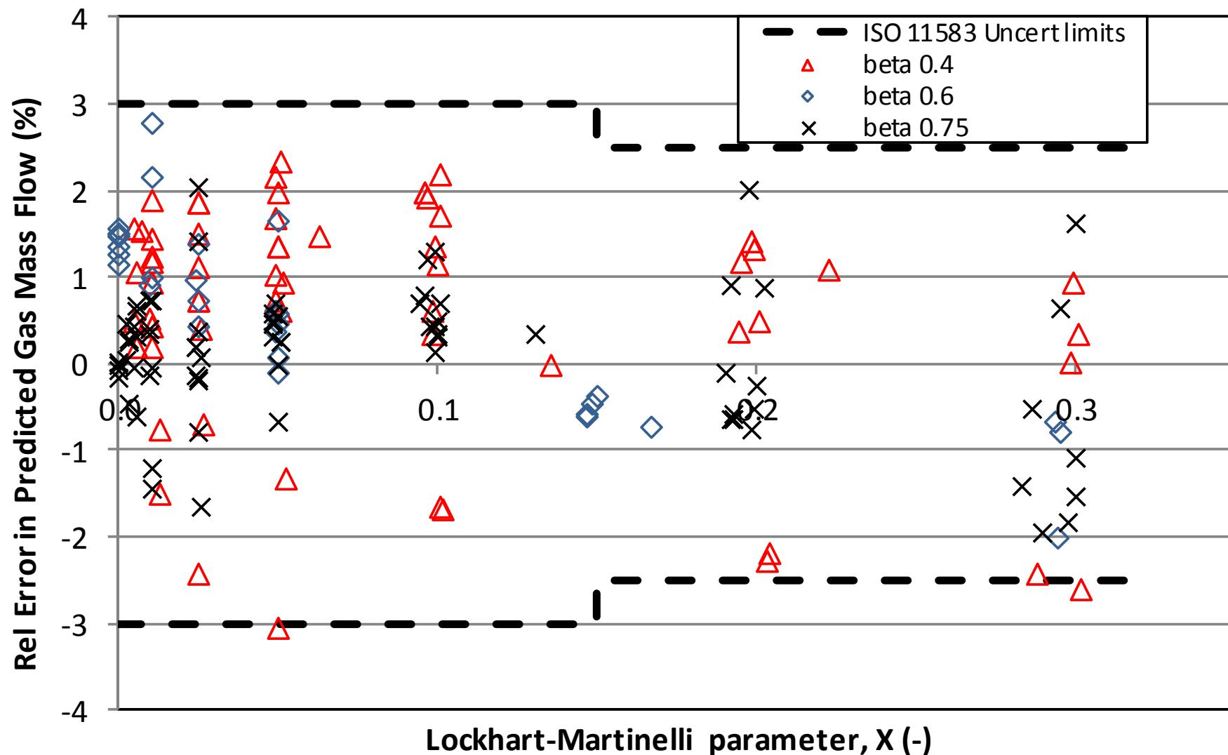
Using fitted values of  $n$  for each Venturi and using either wet-gas discharge coefficient from ISO/TR 11583:2012 or dry-gas discharge coefficient
